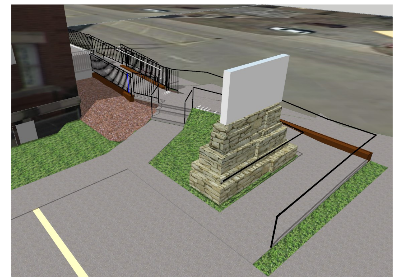
Exterior Ramp Configuration from Parking Lot
